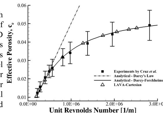
Figure 3: Comparison of numerical, analytical, and experimental results for flow through PIA-C-7020D.
