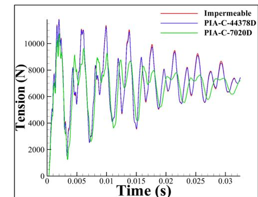
Figure 5: Comparison of the computed tension in the suspension lines for three different parachute canopies in  $M=2.2$  flow. The average force is reduced by  $\sim 7\%$  between the impermeable and PIA-C-7020D canopies. Thus, there is a tradeoff between aerodynamic drag performance and stability (it is commonly known that more porosity = more stability, until  $\sim 80\%$  porosity).
