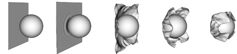
Figure 2: Demonstration of the LAVA-Structural solver on a highly nonlinear contact/impact problem with soft goods.
