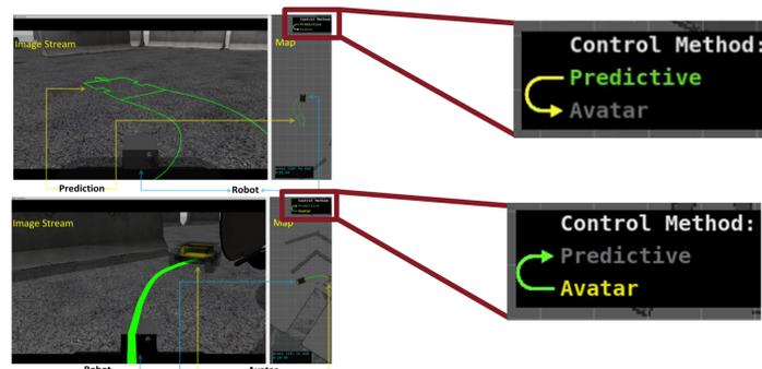
Hybrid interface: the operator has the option to change between PI (Predictive) and AAI (Avatar) at any point of the task. Active method is highlighted in color and transitions between them are represented with an arrow.
