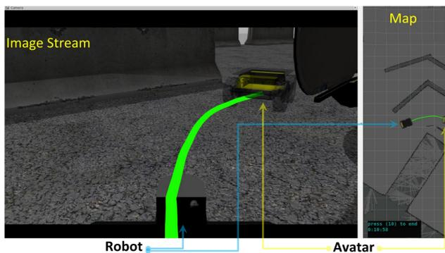
Avatar aided interface with semi-autonomous control: Avatar is augmented on the image stream with some transparency and planned trajectory is represented in green.
