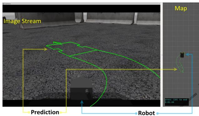
Predictive interface with direct control: The predictive elements (final position and trajectory) are represented in green.
