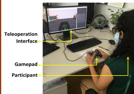
Operator using the avatar aided interface in the context of the experimental apparatus
