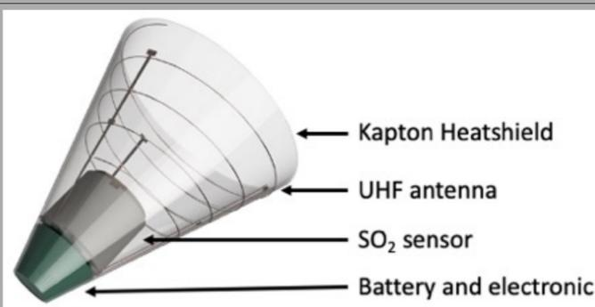
Figure 1: Rendering of a femtoprobe .
