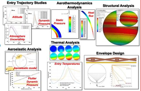
Technical feasibility demonstrated by trajectory, aerothermodynamic CFD, aeroelastic, thermal, and structural FEA analyses & design studies.
