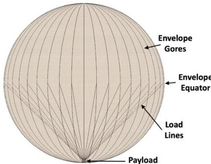
**Packing, Deployment and Inflation.** Packing, deployment and inflation of any space inflatable structure can be a challenge, but the lessons learned in the NASA Echo Balloon Satellite Project point to solutions. There are several options for inflating the envelope including gas stored in high-pressure tanks; subliming solids; or vaporizing liquids. For the NASA Echo balloons, subliming solids inflated the envelope in only 30 seconds using just the heat of vaporization of the solid!
